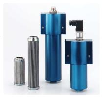
Filters with a bypass utilize elements that are classified as low collapse and can withstand differential pressures up to 450 psid, 30 bar. Filters with no bypass utilize elements that are classified as high collapse and can withstand differential pressures up to 3000 psid or 450 bar. The cost between bypass and non-bypass filter assemblies is minimal, however, high collapse replacement elements can cost up to 300% more than low collapse elements.
