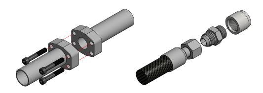
Step 3: Insert Sample Port Fitting into connection using extended bolts (Sandwich Plate models) or existing adapters (T-Fitting models).
