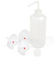
Solvent dispenser with dispensing filters
